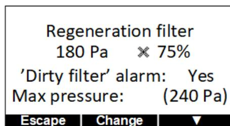
The settings for 'Dirty filter' have the above appearance and, as can be seen, it follows has the same overall structure. The difference is that that the last row, max pressure, presents the pressure level that, if exceeded at given current actual fan speed, will trigger the alarm. A quick comparison of this value, 240 Pa in the example, and the current actual pressure drop of 180 Pa will give an indication of the filter status.
