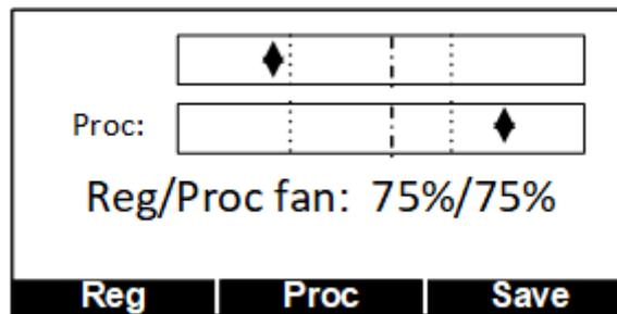
Begin by adjusting the regeneration fan, thus selecting Reg on the lower left button. The machine will now present a screen with the regeneration fan speed highlighted and minus and plus options on the lower left and right buttons. The minus button, lowering the speed of the fan, will move the current actual to the left while increasing the speed will move it to the right.
