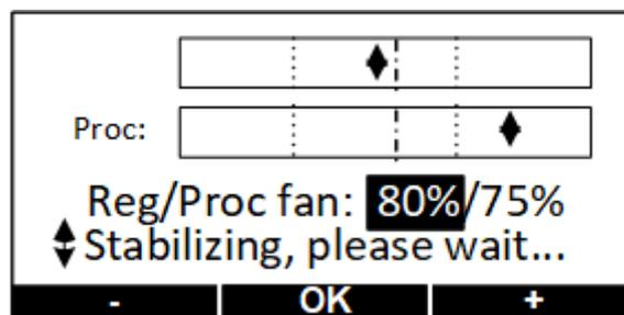
The power developed by the PTC heaters is, as previously described, governed by how much they are cooled with the air flow. Thus, if the temperature of the regeneration air is expected to drop significantly during the operation, it is recommended to leave the regeneration operation point towards the lower end of the allowed interval.
