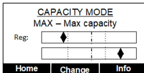
In the example above, the machine is operating in Max mode and both indicators are currently outside their allowed intervals. To adjust the operation, push Change and then confirm the selection of Max mode.
