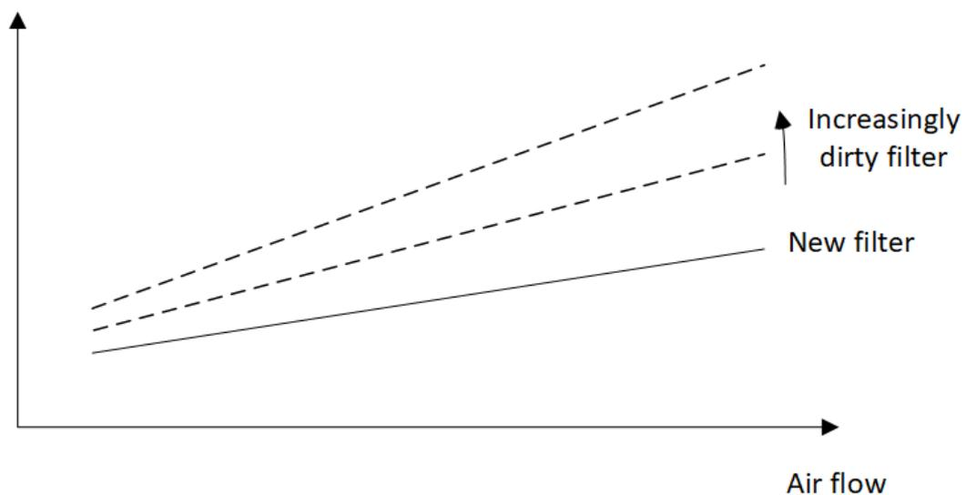
To get the alarms to trigger at the correct point in time with given installation will thus often require the pressure drop settings to be changed. Installations with long ducting will cause the actual air flows to change and, as a consequence, the user might find that the factory settings for the alarms do not quite fit requirements.
