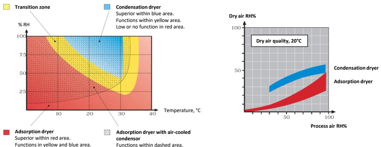
Condensation dehumidifiers are, in accordance with the diagram above, used in hot and humid conditions provided the goal and aim is drying of rooms, ambient air.
