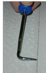
Fig. 32 Manual test with seam probe
