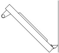
Holding the door on both sides, lift door back up to 45° and carefully pull the door out and away from the hinges.
