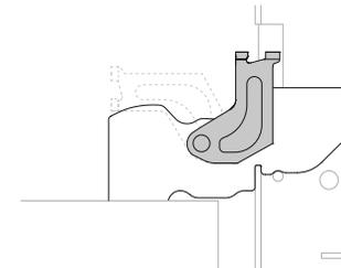
Rotate the locks up into the closed position ensuring they rest inside the slots completely. Note: Incorrect installation will prevent door from correctly sealing.
