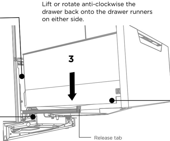
Lift or rotate anti-clockwise the drawer back onto the drawer runners on either side.
