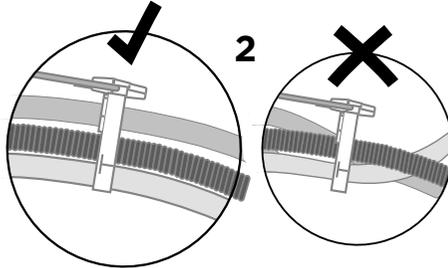
Before refitting the drawer, ensure the hoses are not twisted and the latches at the rear of each drawer runner are facing forward.
