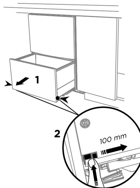
Press the release tabs in on either side and push back to release drawer from runners. Lift drawer off runners.
