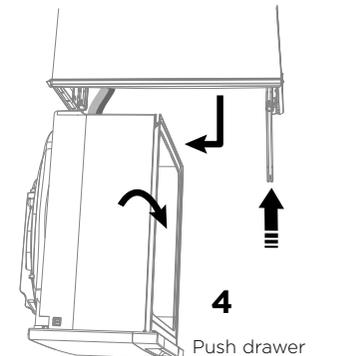
Rotate the drawer clockwise (max. 90°) and rest on side.
