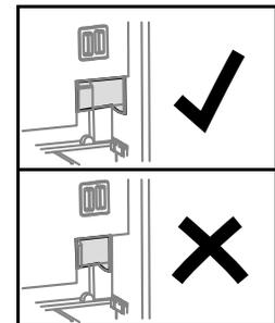
Pull the release tabs forward on both sides 100 mm. Ensure the tabs are fully pulled forward and click into place.
