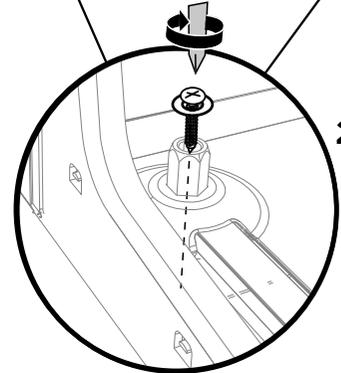
a pair of fixing holes either side on the bottom (use 38 mm fixing screws & washers)
