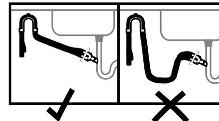
Ensure drain hose is routed straight to the joiner so that waste water does not accumulate in the hose. Remove excess drain hose material if necessary. Do not shorten the inlet hose.
