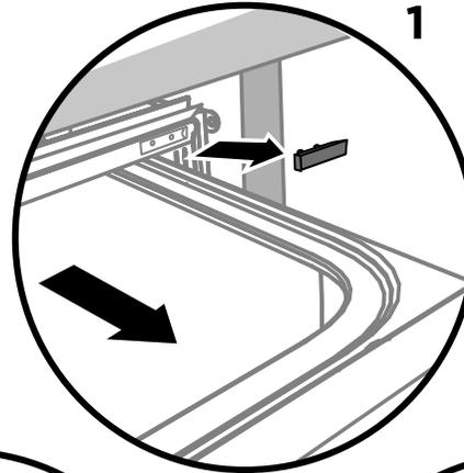
Open the drawer halfway. Using a flat bladed screwdriver, prise the grey rubber plug out of the trim moulding.
