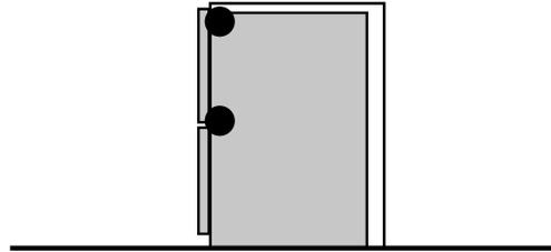
**8-A ATTACH SIDE MOUNTING BRACKETS**
