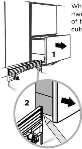
Where the toekick meets the bottom of the tub is the cut-off point
