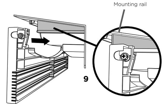
Slide the toekick onto the mounting rails either side and screw the toekick onto the bottom of tub on either side.
