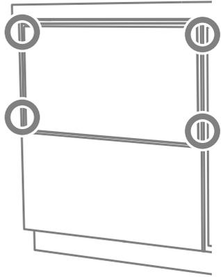
Using a small Philips screwdriver, screw through the trim moulding, securing the side mounting bracket to the cabinetry. Do not damage the rubber trimseal.
