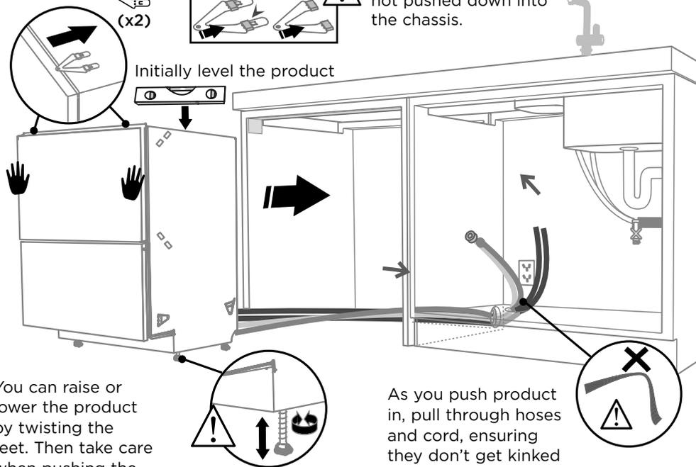
You can raise or lower the product by twisting the feet. Then take care when pushing the product into the cavity that you do not bend the feet.
