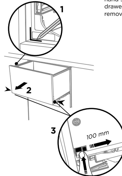
Press the release tabs in on either side and push back to release drawer from runners.
