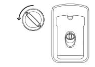
Turn the cap anticlockwise and remove.
