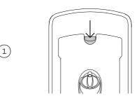
Press the latch down to open the dispenser. Check that the dispenser is empty and dry.
