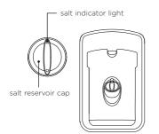
The salt reservoir is located on the inside of the drawer next to the detergent dispenser. It holds up to approximately 350g of salt (actual capacity will vary depending on brand and grain size of salt used).
