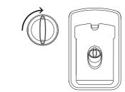
Refit the cap, turning clockwise until secure.
