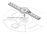
Lift the spray arm off the impeller. Shake to dislodge any loose particles, rinse under running water and wipe with a damp cloth.
