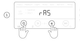
Ensure there is no wash in progress. Press and hold and  $\bigstar$  together for 4 seconds to enter the menu.
