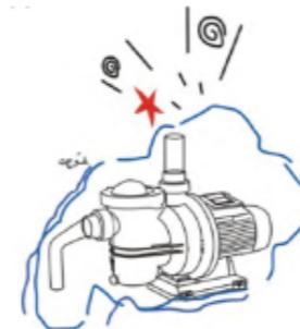
**EN** Low flow rate: low pressure in the filter.
