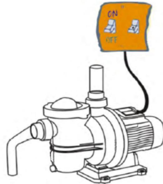
**EN** Fill the pump, slowly and completely opening the gate valve in the suction pipe, and keeping the gate valve on delivery open to let the air out.
