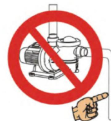
**EN** Suction pipe diameter > = diameter of the electro pump opening.
