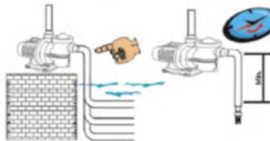
**EN** If there are several suction pipes, arrange the pipes and the manifold below water level and reach the pump with only one vertical pipe.
