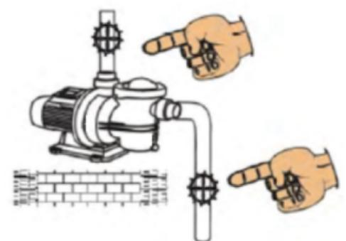
**EN** Fit one gate valve in the suction pipe and one in the delivery pipe to isolate the pump.
