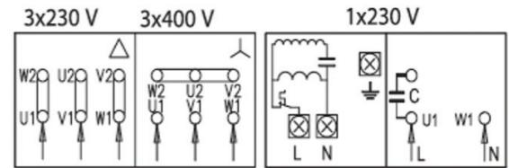
**EN** Voltage must be the same as shown the motor plate.
