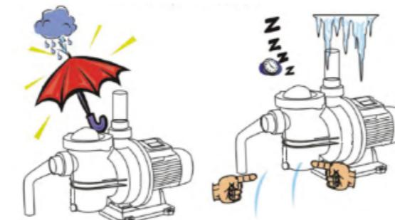
**EN** For long periods of inactivity or frost, remove all the caps and completely drain the pump body. Keep the caps!
