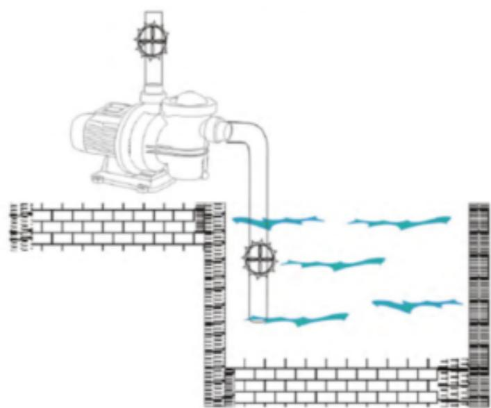
**EN** The pump is able to overcome a maximum difference in level of 1,5 m.
