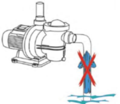
**EN** No water in the prefilter or clogged prefilter.
