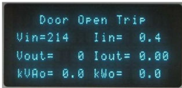
Figure 12: Display showing Door Open Trip
