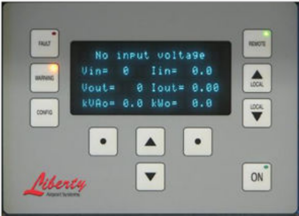
Figure 18: Typical Warning Message - No Input Voltage
