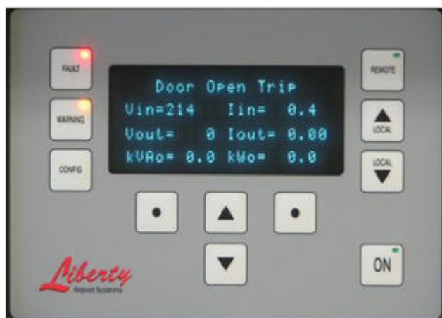
Figure 19: Typical Fault Message - Door Open Trip
