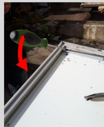
[C] use a flat screwdriver to lever the profile out of the frame
