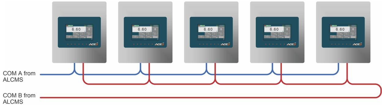
Using the recommended Belden 9842, the communication should be terminated using the example below.
