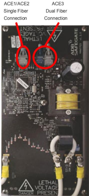
The CVM2 is the latest generation monitoring module. This module is backward compatible with all previous versions of CVMs and can be used as a direct replacement.
