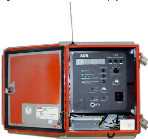
Figure 1: L-854 Radio Control Equipment
