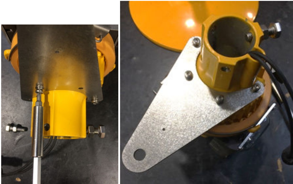
Figure 40: Mounting the Support Plate
