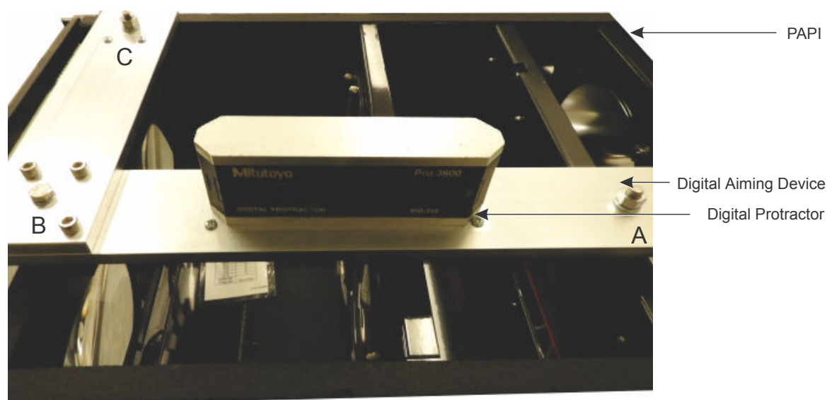
Figure 12: Side View of Digital-Level Aiming Device for Two-Lamp PAPI
