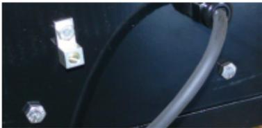
Attach the earth ground lug if not present. The earth ground lug is located on the outside frame of the sign to permit easy connection of an AWG 12 (minimum) earth ground wire to the sign.
