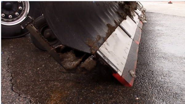
Fig. 1 - Snowplow blade with well aligned segments
