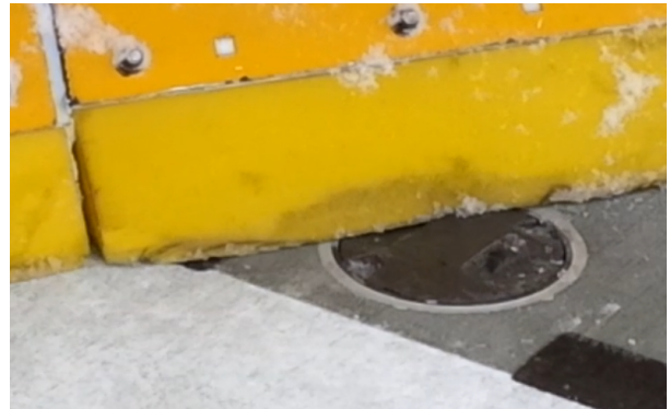
Fig. 3 - Snowplow blade without clearance
