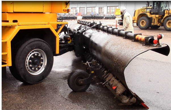
Fig. 4 - Snowplow with support wheels
