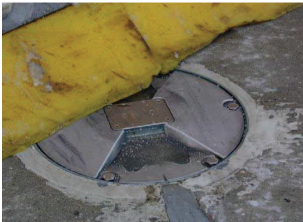
Fig. 2 - Snowplow blade with wear and steps between segments
