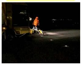
FB Tech has developed a cleaning system that can be either installed in a vehicle or on a trailer allowing for rapid intervention, and in difficult climatic conditions.
