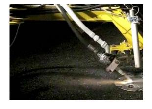
The equipment can be installed inside the Airport maintenance vehicles that will pull a compressor 7bars/ 5000litres or on a specifically designed trailer where compressor, the dry-ice container and the machine are fitted. Contact us to define your requirements.
