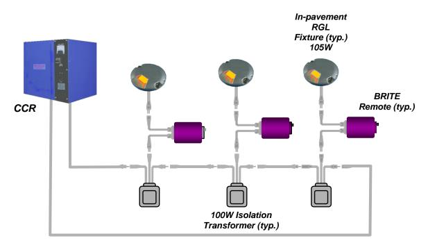
Figure 1: Un-monitored in-pavement RGL system.
