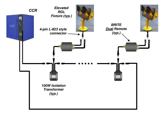
Figure 2: Un-monitored elevated RGL system.
