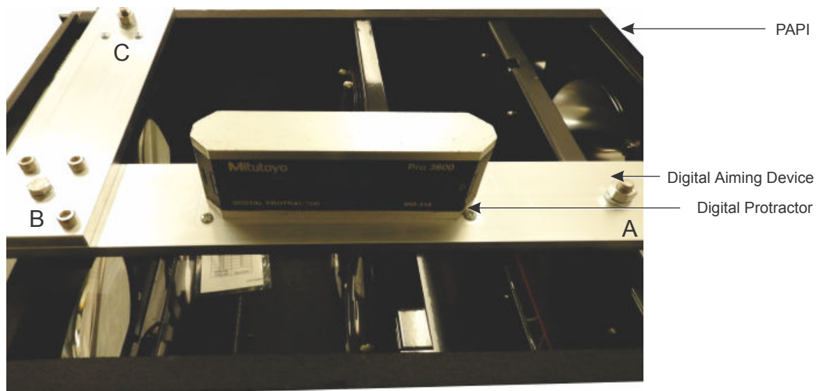
Figure 10: Side View of Digital-Level Aiming Device for Two-Lamp PAPI
