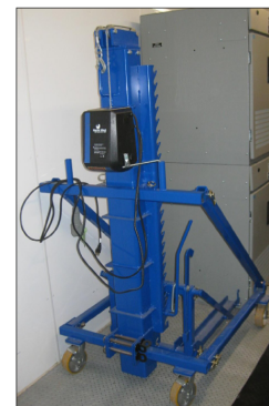
1" Power Lift next to Switchgear Regulator Assembly.
