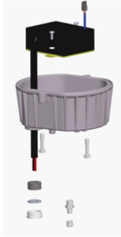
Figure 6: SL-TE-I VAC converter removal
