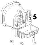
**F)** Connect the lamp on the cable terminal.
