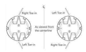
Triangle embossed on the top cover should point toward the centerline to ensure correct toe-in position.
