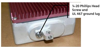
Figure 3 Field Lightning Arrestor Ground Screw
