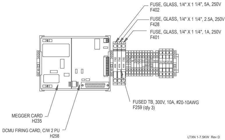
**Figure 22: 1 - 7.5 Component Plate**
