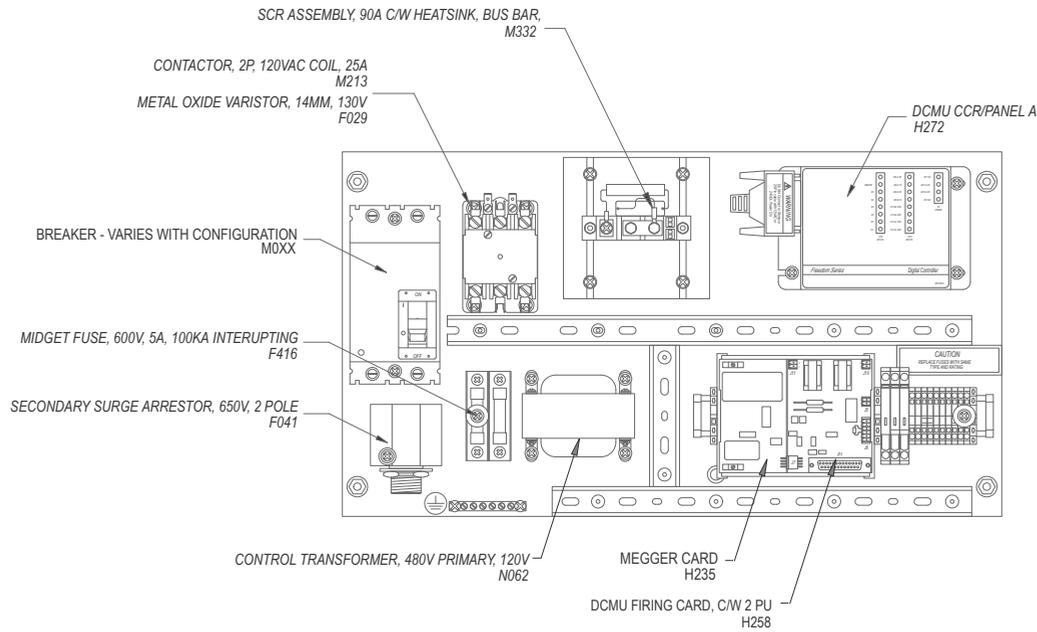
**Figure 24: 20 kW Component Plate**
