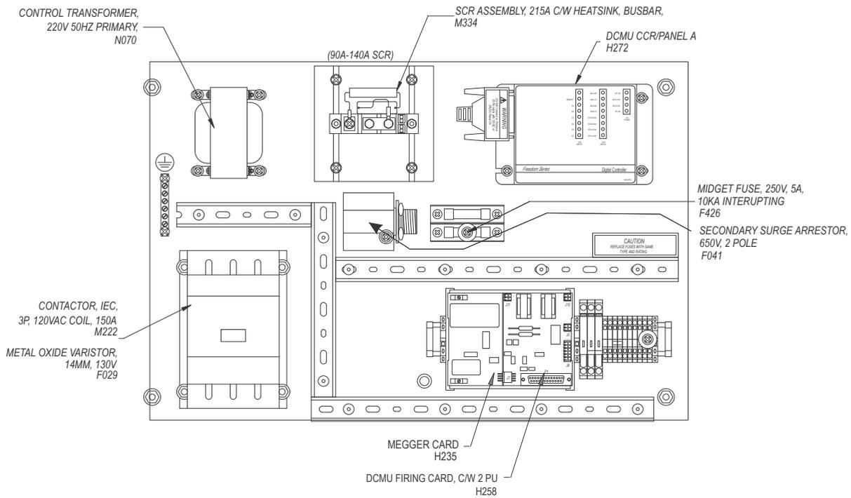
**Figure 25: 30 kW Component Plate**
