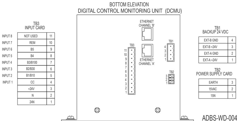
**Figure 7: DCMU Connections for Alarm and Safety**
