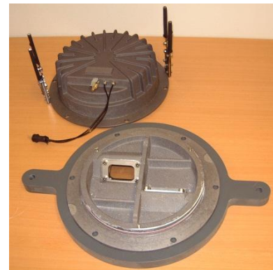
FIGURE 4 – REMOVING THE INNER COVER
