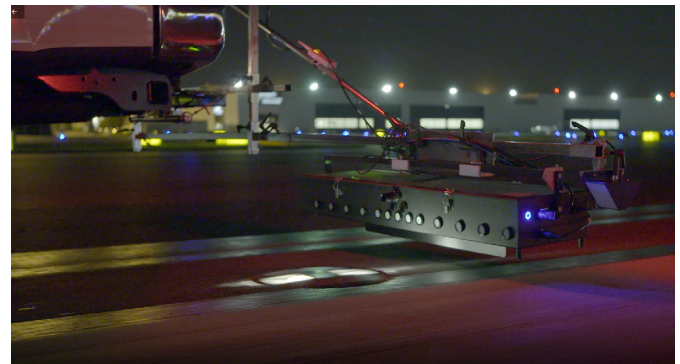
PAC Light Sensor has sensors on front and back of the sensor strip requiring only a single test pass over the light fixtures cutting testing time by 50%.
