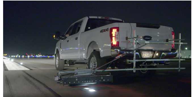
Mobile PAC can be used with any vehicle and installs easily with portable frame onto standard 2" trailer hitch.
