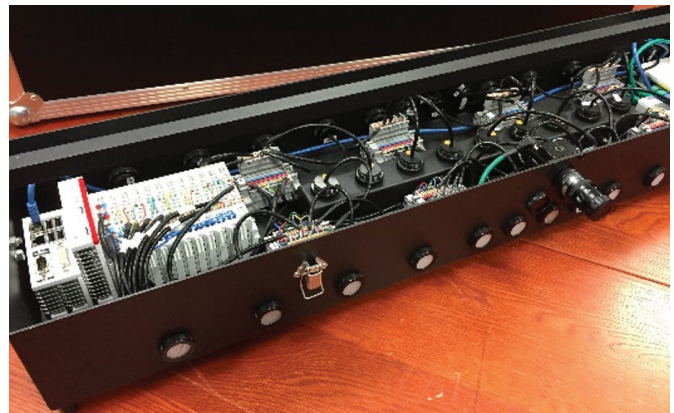
PAC sensors strip contains the PLC.
