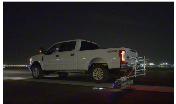
PAC Mobile easily measures photometric data of Inpavement and runway elevated lights assuring compliance with FAA and ICAO standards.
