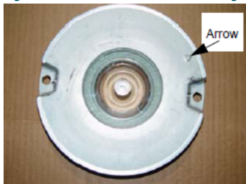
Figure 13: Index Pin of Inner Cover Flange
