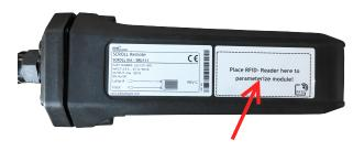
The orange connection waves symbol on the reader indicates where the RFID antenna is located, i. e. where the reader must be held in front of the remote to establish a connection.
