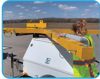
2. Extend the 4 light assembly arms
