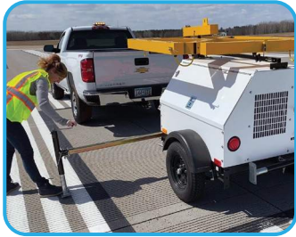
1. Level as necessary using 3 leveling jacks
