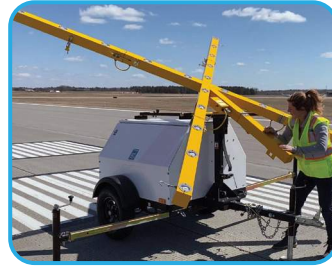
3. Tilt the light to the upright position
