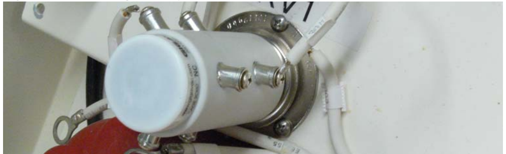
Figure 13: Mounting the relay
