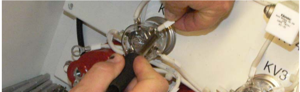
Figure 7: KV1 being de-soldered
