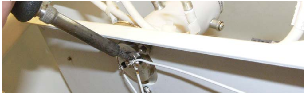
Figure 14: Solder the wires and diode
