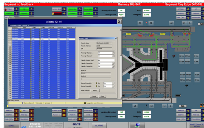
ATC activation and display of dedicated taxiing routes with ALCS Style 7 and individual aircraft guidance via AGLAS® lamp control
