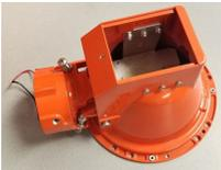
5. Remove four (4) #8-32 X 1/2 in phillips head screws (64A0191/8), four (4) #8-32 nylon insert lock nuts (65A0347/8), and two (2) black nylon hole plugs (63A1091) holding the LED light engine in place and discard.
