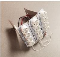
6. Insert the new LED light engine into the flash head ensuring the leads are at the bottom of the LED light engine. Attach using new hardware: four (4) #8-32 X 1/2 in phillips head screws (64A0191/8), four (4) #8-32 nylon insert lock nuts (65A0347/8), and two (2) black nylon hole plugs (63A1091).
