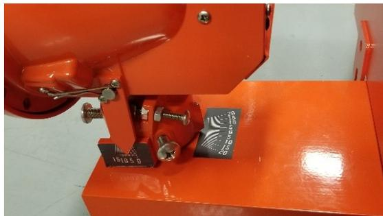
2. Hand-tighten all 3 screws and jam nuts when adjustment is completed. Check the alignment pointer to verify that the required horizontal angle is correct. Repeat the adjustment procedure if the angle is not correct.
