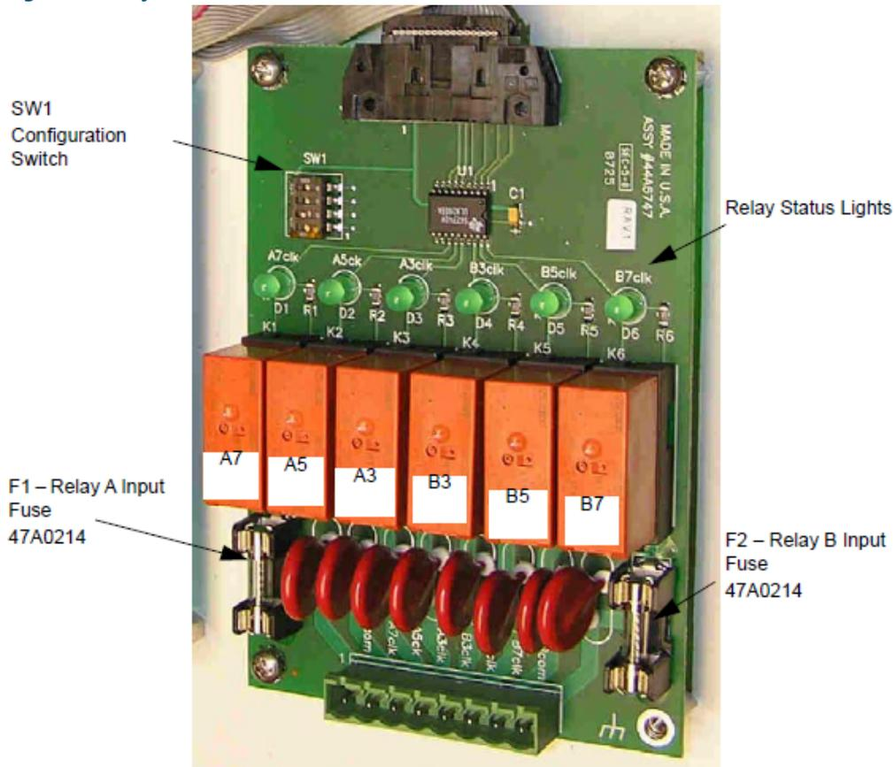
See Figure 5. The Radio Control Equipment provides for relay outputs for control of external lighting. Either of the two relay sets can be configured for either cumulative (incremental) or, individual output. See Figure 4 and Figure 5 for a description of the logic used. All relay contacts are dry, and can switch either +48Vdc or 120Vac through either set of relays for CCR control.
