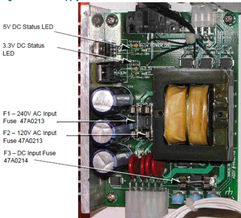
See Figure 4. The Power Supply board provides 5 VDC and 3.3 VDC to the various boards in the system. Input power is brought in through the (see Table 4), Terminal Block at the bottom of the cabinet. Input power options include:
