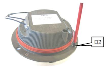
4. Introduce the special opening tool (see page 46) or a flat screwdriver in the dedicated slot between cover and inner cover and rotate it to separate the inner cover from the cover.
