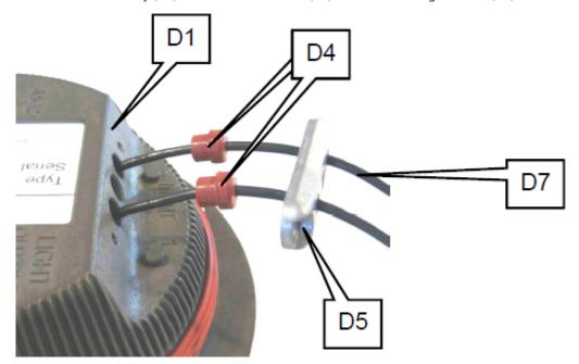
6. Bring the new ADB cable assembly through the wire clamp (D5)
