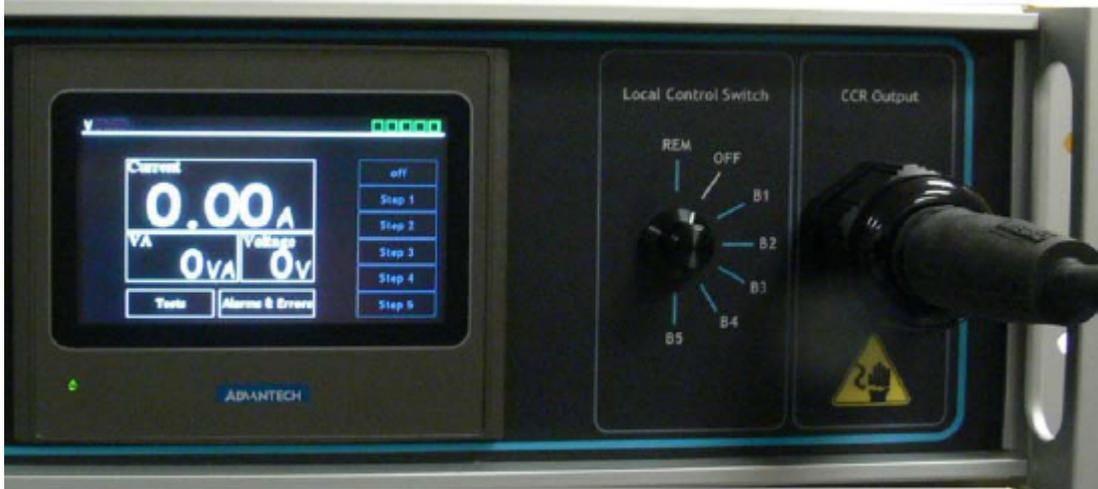
Manually select the desired output by setting the rotary switch to B1 through B5.
