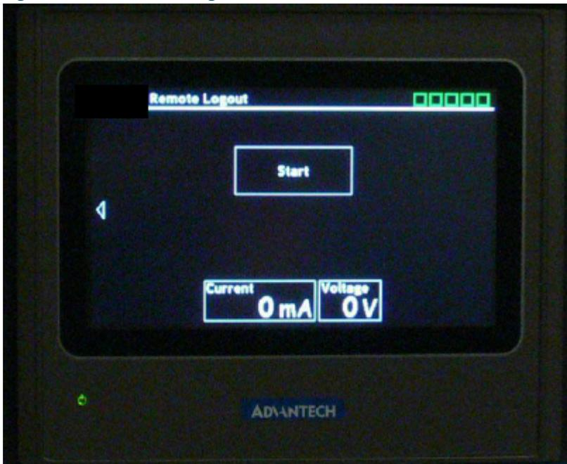
This screen can be reached by pressing the "Remote Logout" screen on the Test Scenarios screen. A separate box is used to connect the CCR to the Remote. Contact the ADB Sales Department for further details.
