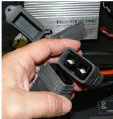
Power Inverter 12 VDC Coupling.
