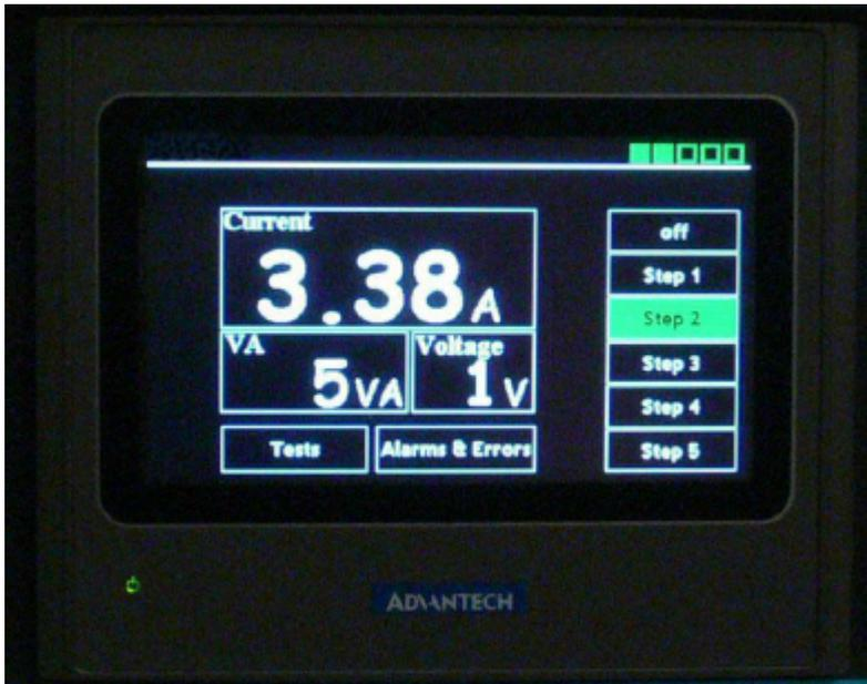
Pressing the alarms & errors button on the main screen will take you to the Alarms & Errors screen.
