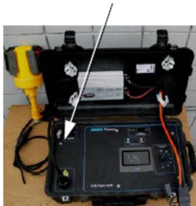
Light connected, power inverter ON, Field CCB circuit breaker ON and rotary switch OFF.
