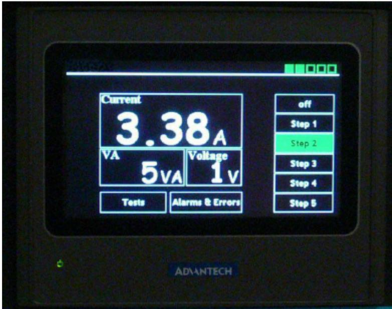
You may adjust the Requested Step field and use the arrow keys to select the desired 5-step current steps to apply to the output.
