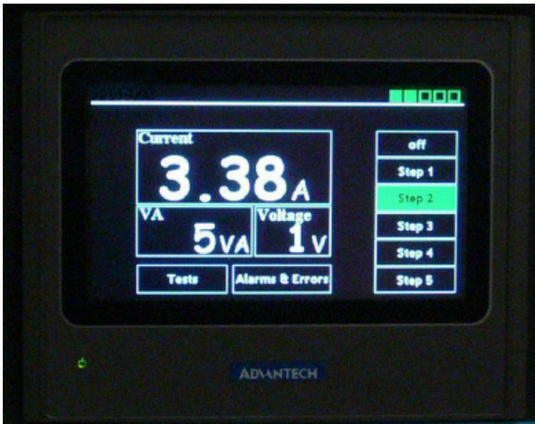
From this screen you can view the current, VA, and CCR output voltage and watch the values in real time.
