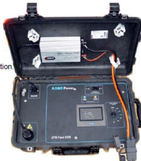
8. Connect the airfield light to test.
