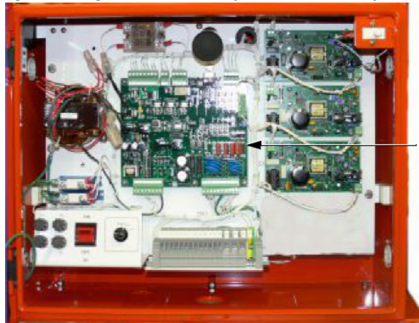
Figure 12: Voltage Powered LED REIL, Style A/E Interior Assembly
