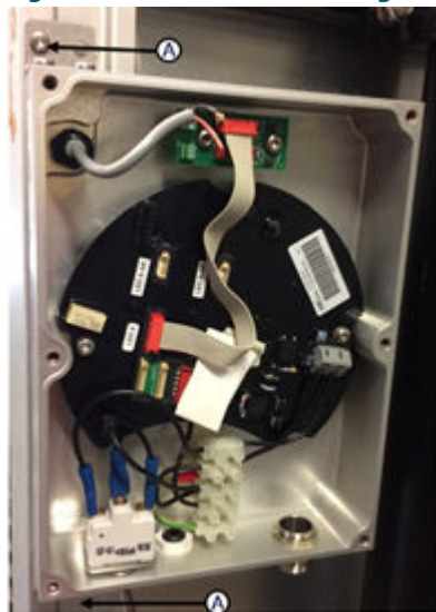
Figure 36: Electronic Box in Sign Frame
