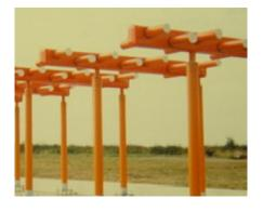
EXEL localizer supports are full scale impact tested, lightweight and practically maintenance free.
