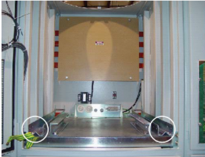
Figure 35: Empty Upper Powerpack Bay
