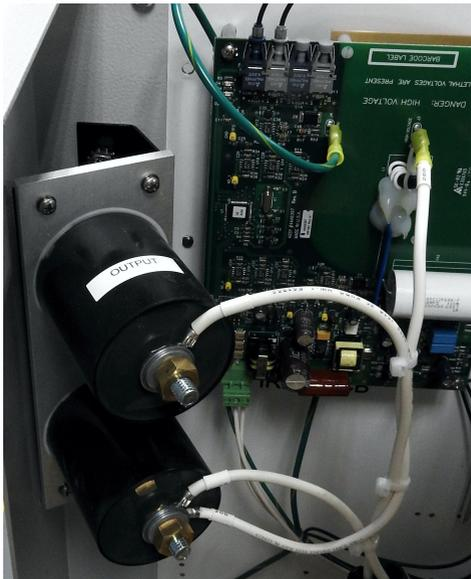
5. Loosen the 11/16-inch wire retaining nuts for 200, 201, 203, ST1, ST2 and 202 and disconnect.
