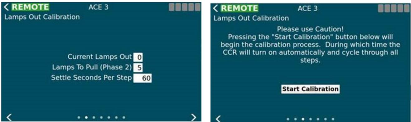
The calibration consists of two phases. The first is calibrating the existing circuit. The second is pulling a set number of lamps and calibrating again.
