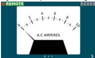
This view is shown when the ACE3 mode is "CCR" and the display mode is L828 or when the "Display Analog Current Gauge" feature is enabled.
