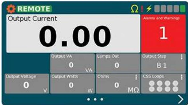
The main screen is the first usable screen (not the splash screen) the user sees after starting the ACE3 (except when in L828 Display mode). The page is laid out with a header at the top and the body below it. The body contains a large display which shows the primary item being monitored.
