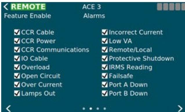
Disabling an alarm or warning prevents that alarm/warning from showing up on the alarm page and the corresponding event(s) will not be generated.
