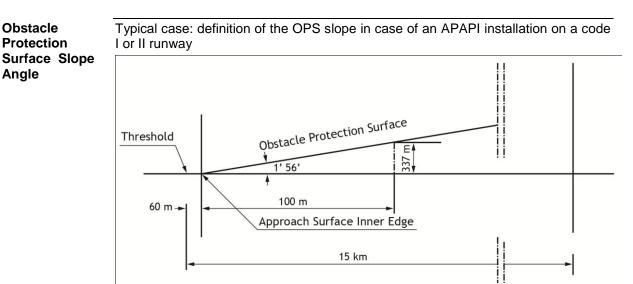
The slope of the surface can be calculated by the following formula:  $\theta 2 - 0.9^{\circ}$ .
