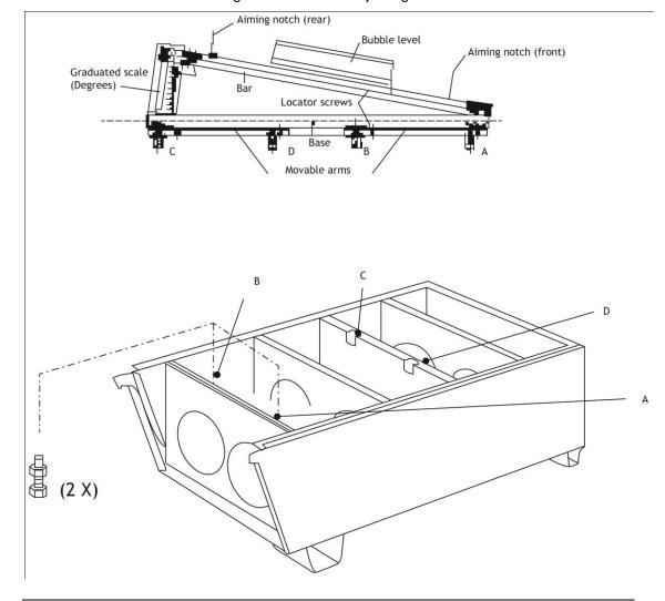
**Aiming device** This illustration shows the aiming device used for adjusting the units in elevation.
