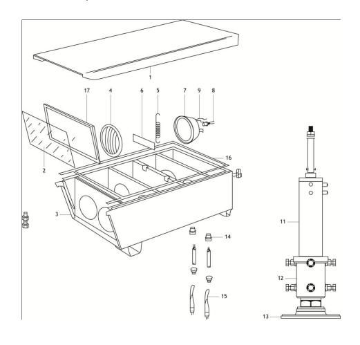
PPL 400/3 Below is the exploded view of the PPL 400/3 PAPI unit.
