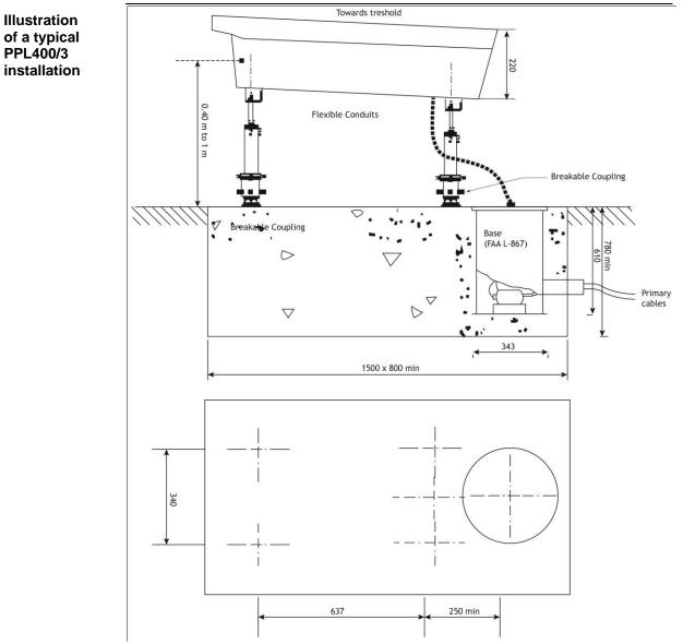
Note : the FAA L-867 base can also be replaced by conduit elbows leading, via conduits, to a transformer housing installed further away from the PAPI unit.
