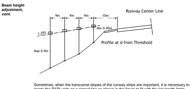
Sometimes, when the transverse slopes of the runway strips are important, it is necessary to locate the PAPI units on a sloped line as shown in the figure to fit with the leg length limits, while keeping the four PAPI units aligned on a same perpendicular axis to the runway.
