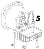
**F)** Connect the lamp on the cable terminal.
