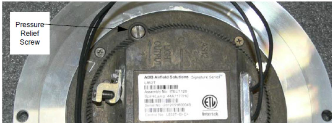
**Figure 29: Pressure Test Fitting Assembly**
