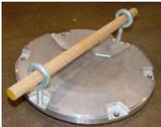
The lifting tool can be made from two 1/2 x 13 eyebolts (1-inch ID) and a 1/2-inch diameter, 16-inch (406mm) long rod or pipe inserted through the eyebolts.
