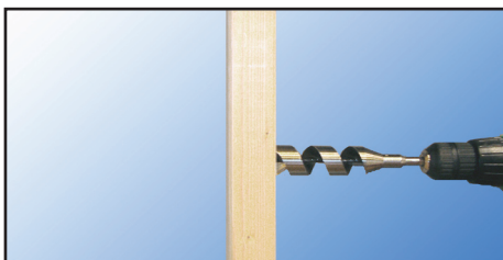
Bor 32mm hull i stender.
