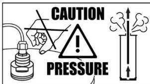
**WARNING: CHECK THAT THERE IS NO WATER PRESSURE. Otherwise the quartz tube could be ejected from its housing!**
